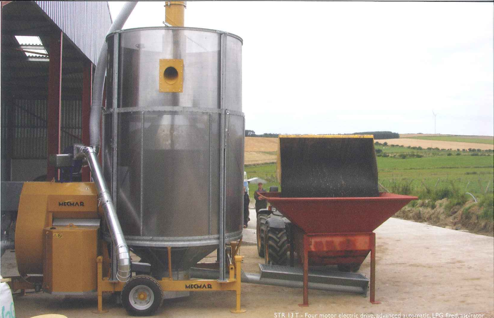
STR 13T - Four motor electric drive, advanced automatic, LPG fired, aspirator
